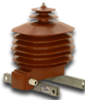
Phase to ground connected, epoxy insulated voltage transformer 19/0.11kV
